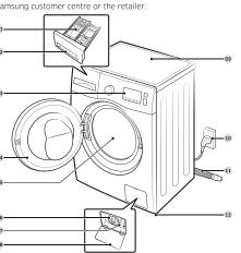
**05** Drum 06 Pump filte 07 Emergency drain tube 08 Filter cover 09 Worktop
