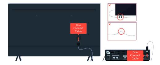
Disconnect and reconnect the One Connect cable between the TV and the One Connect (OC) Box. Make sure that the One Connect cable is not pinched or bent sharply.
