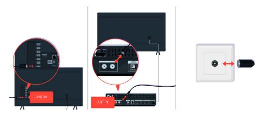
Check the antenna and input cable connections.
